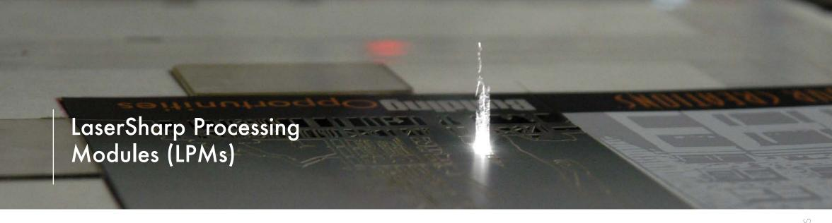
**LPM1:** A fixed beam enables repeat and registered down-web scoring and precision perforating for easy opening. Applications include:
